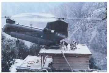
He showed a picture of an unusual military heliport, where the rotors must keep turning to lift the front of the helicopter an angle to set down the tail ramp.
