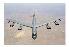
Another bomber, the B-52, was of considerable size. Unlike most bombers designed to avoid radar by flying at high altitude, the B-52 was able to fly at very low altitude to avoid ground radar.
