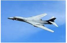
The B-1 bomber was created as a newer, much more sleek, and versatile bomber. Like the B-52, the B-1 was designed to fly at very low altitudes, and the plane featured new terrain radar technology that could draw out terrain heights for safe flying at low altitude. However, even more significant leaps in innovation were to come.
