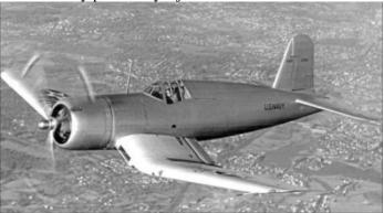
Vought XF4U-1 Corsair fighter prototype, which Trap flew at 402 mph in an official Navy speed trial
